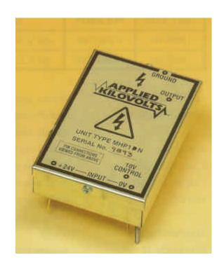
This range of power supplies are miniature versions of the HP family giving up to 1kV, 2.5kV, or 3kV, at 2W. The units, which are programmable by a 0 to +10 volt signal, are intended to be mounted on a printed circuit board and offer high stability together with low drift. They use high frequency pulse width modulated switching techniques in conjunction with a ferrite step-up transformer to control the output voltage.
